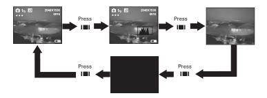
In the Playback mode, press the Display button once to show the information display with a histogram. Pressing the button again will turn off the information display on the LCD screen, with nine thumbnail picture and video clip files left only. Pressing the button a third time will show a picture or video clip file in full screen with the information display.
